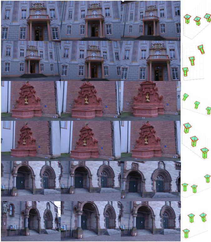
Fig. 9. Trifocal relative pose results for EPFL dataset. Each row shows images with ground truth (green) and estimated poses (red outline).
